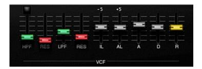
ME 80 has 2 filters for each synthline. A high-pass and low-pass filter together will sound like a band-pass filter. The filters are 12Db/octave.
